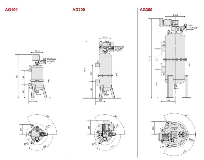
The inlet and outlet nozzles can be turned one toward the other (180°, 90°,...)
