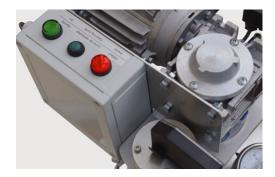
**Filtration.** Filtration is achieved through a cylindrical screen. As soon as the filter screen is clogged, a pressure switch detects the pressure difference between inlet and outlet and starts the cleaning cycle.
